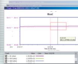
(新架構) 高速洩漏電流偵測 應用範圍: 離子遷移、CAF (New infrastructure) High-speed detection of current leakage Applicable scope - ion migration - CAF
