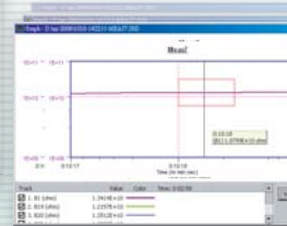
(新架構) 高速洩漏電流偵測 應用範圍: 離子遷移、CAF (New infrastructure) High-speed detection of current leakage Applicable scope - ion migration - CAF
